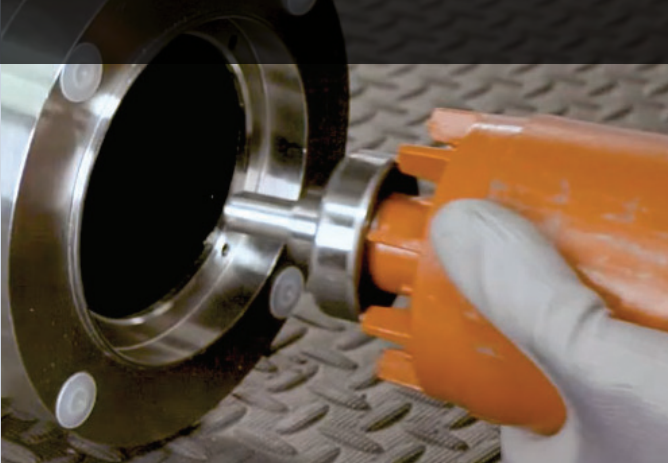
3. Insert new O-Car™ into motor shell.
