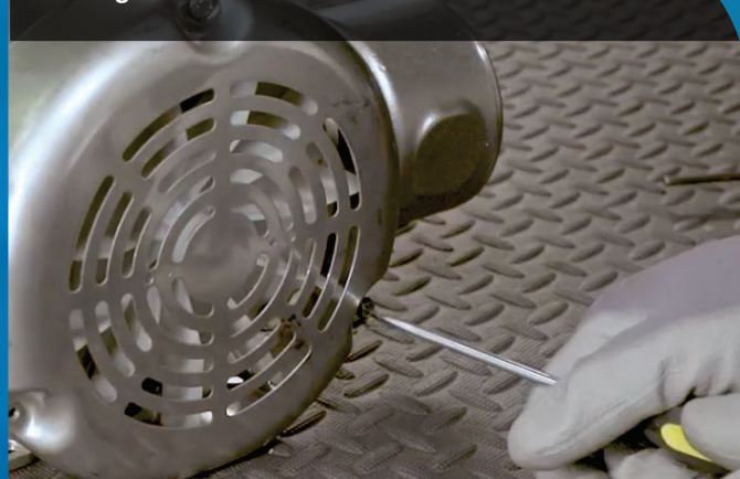
4. Reassemble external fan, retaining ring, fan guard and screws to motor.
